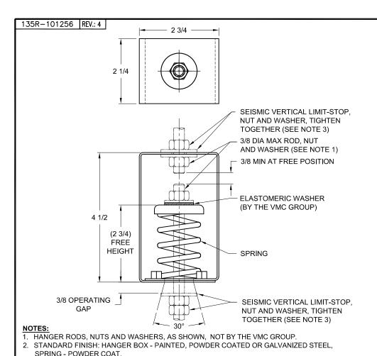
SEISMIC VERTICAL LIMIT-STOP REQUIRED FOR SEISMIC APPLICATIONS. NOT BY THE VMC GROUP. INSTALL WASHER .1 THK, MIN. X 1-1/4 O.D. MIN. WITH REQUIRED INSIDE DIAMETER TO ACCOMMODATE ROD SIZE IN USE. THIS CAN BE ACCOMPLISHED BY USING A SINGLE WASHER OR BY STACKING NOT MORE
